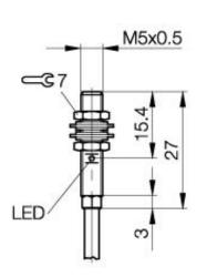
**Inductive Sensors** BES 516-3023-G-E4-C-PU-02 M5x0.5 x 27 normally-closed Sn=1,5mm shielded
